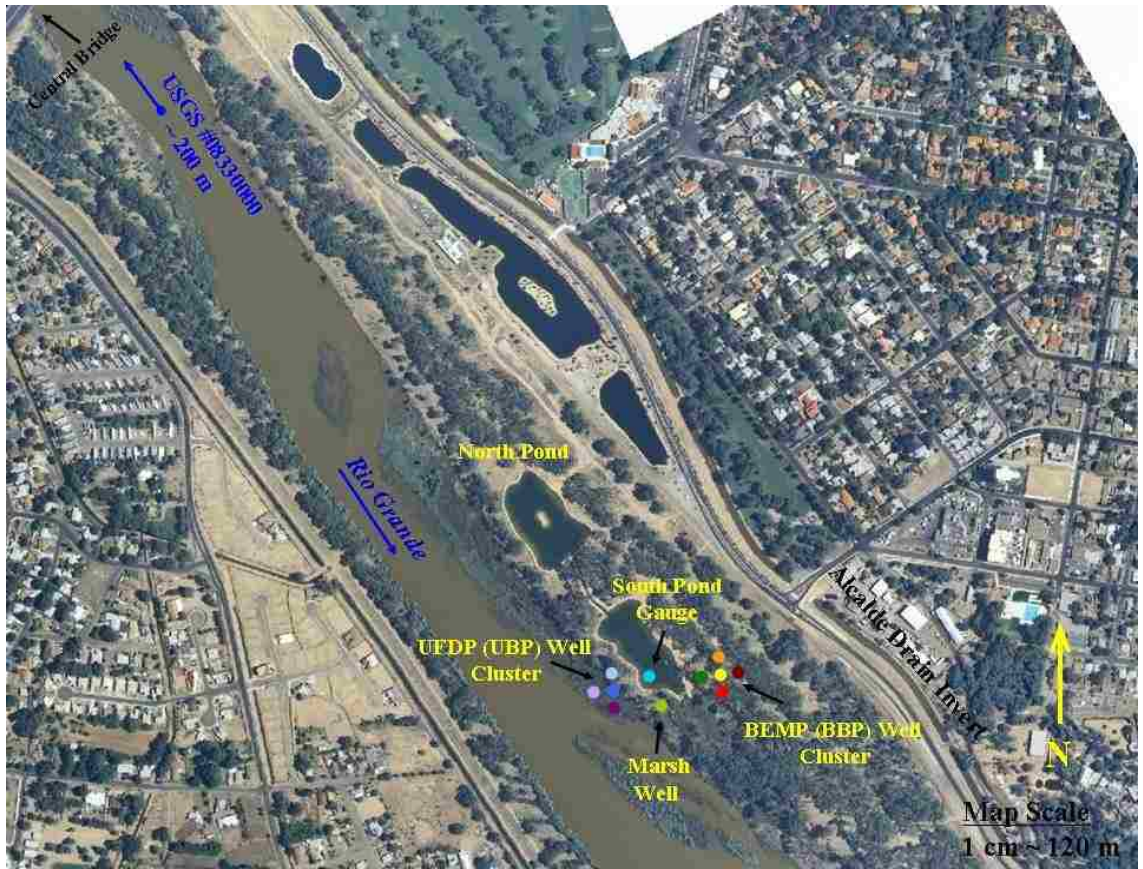
Figure 26 : Location of Biopark ground water monitoring wells (Lejuene & Crawford, 2008). The Colored dots indicate wells.
